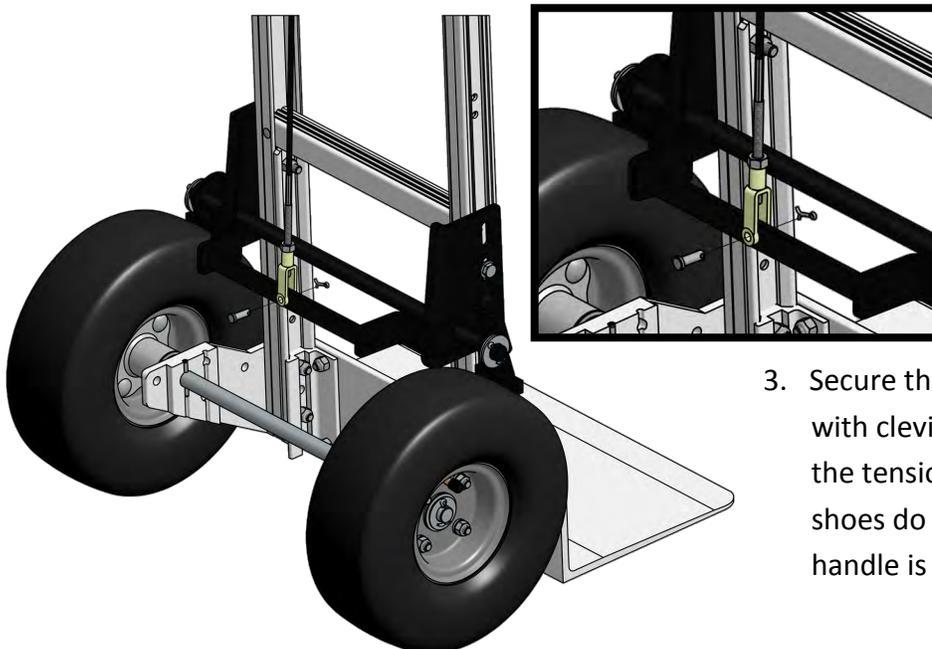
2. Thread nut (D) and yoke (G) on to the end of the cable assembly, threading until the yoke end aligns with the lower brake pull bar.
