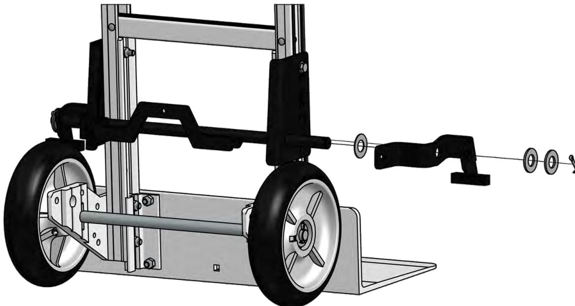
4. Slide the brake shoes apart enough to insert the pull bar (L or M) between the mounting tabs on the brake shoes. Then secure the right side of the brake axle with a cotter pin (K).
