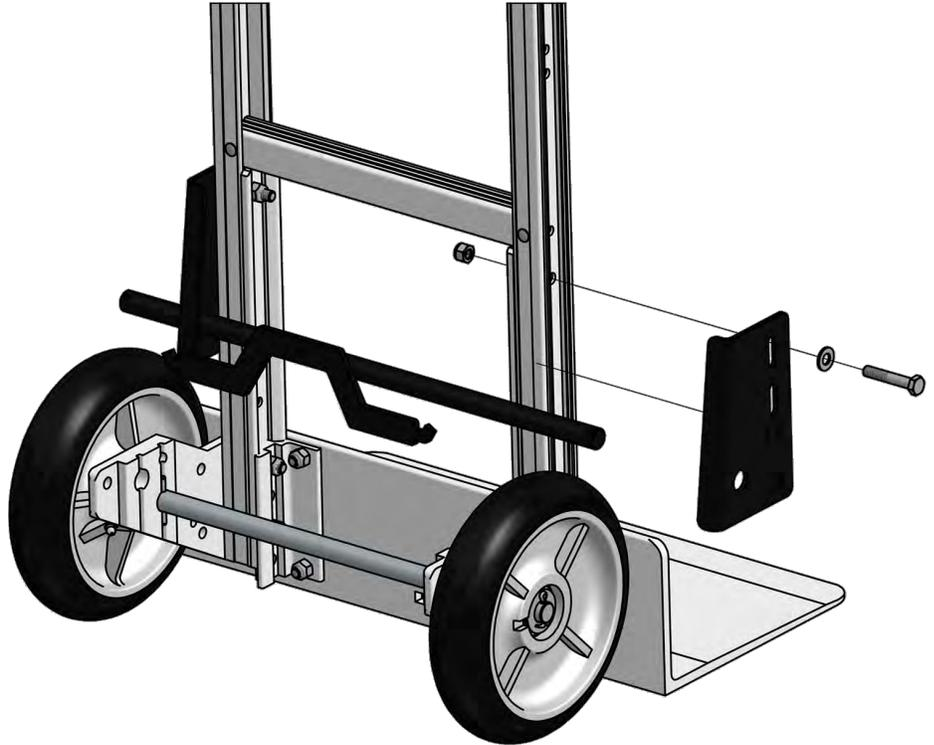
2. Attach the RH and LH brake mount plates (C, D) to the outside of the frame, mounting through the upper stiffener channel with nuts (F) and bolts (J), do not tighten completely. For 8" wheels use the upper slot in the mounting plate, for 10" wheels use the lower slot.
