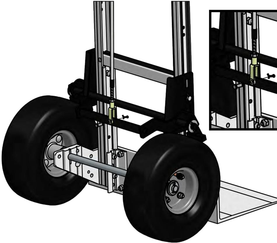
3. Thread nut (D) and yoke (G) on to the end of the tee handle (A), threading until the yoke end aligns with the lower brake pull bar.
